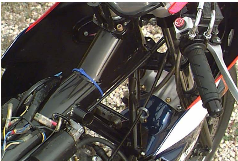
A good look at the 3" main backbone, and heavily triangulated and gusseted steering head. The VF500 swingarm is about 2.5" longer than the stock 400F arm, but the distance between the swingarm pivot and the front axle is about 2" less. The result is a much more modern 56.5/43.5 F/R weight distribution.
