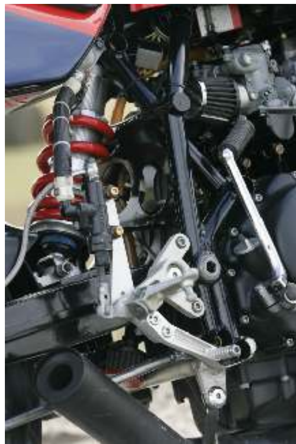
Below - At the rear, a Fox Factory Twin Clicker from an NS400, fitted with an NT650 Hawk spring separate the VF500 swingarm from the custom frame. Hours of machining and multiple set-ups resulted in adjustable rear sets.
