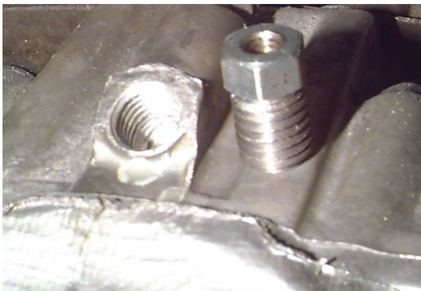
The internally threaded coupling nut was available from McMaster Carr, I machined the outer surface round, and then threaded \frac{1}{2} -13 threads on it, and a matching set into the crankcase. The plug will be “JB Welded” into the case for what should be a permanent, leak proof repair.
