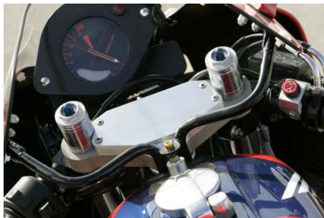
Above - Fabricated parts in this shot include top triple clamp, clamp/fuse box cover, clip-ons, fairing brace, kill switch mount, instrument panel in aircraft grade carbon fiber.
