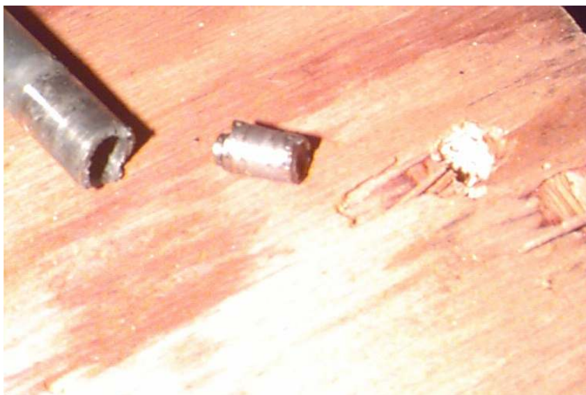
The end of the “holesaw”, and the cored bolt still encased in aluminum
